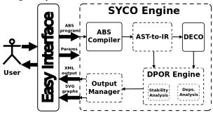
The web interface of SYCO is available at costa.ls.fi. upm.es/syco. Essentially, once the input program is ready, either selected from the available library of ABS programs or supplied by the user, a set of parameters are provided (or just left with bydefault values), the SYCO engine is run and the output is obtained.
